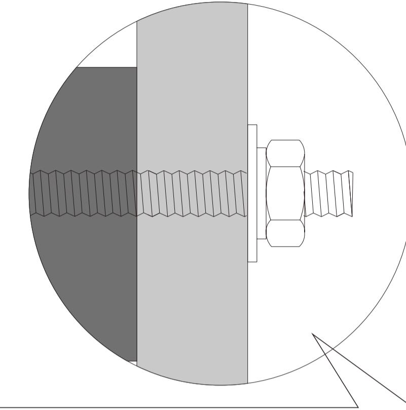
If the backing wall is thin and construction can be performed on the another side of the back wall, please use nuts and washers to fix the stud bolts on the back wall, so that the signage can fix on the backing wall more secure.
